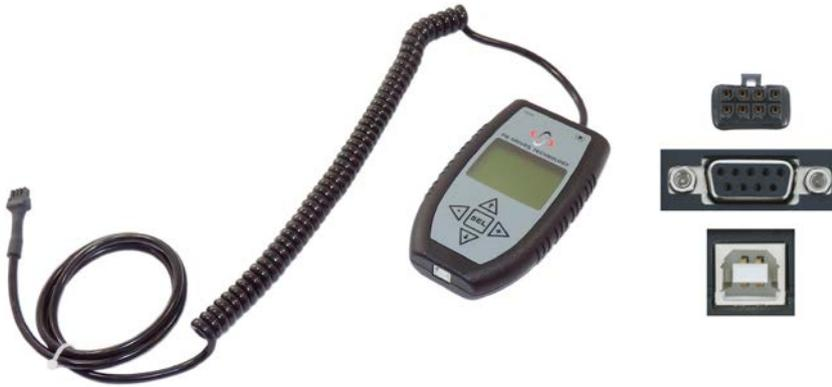
The Sigmadrive handheld programmer is a powerful programming tool used to configure all Sigmadrive controllers and the Sigmagaugage LCD vehicle display. It allows simple and easy matching of motors to the controllers to produce the desired vehicle driving characteristics. It also has a built-in RS232 interface which allows it to re-flash the Sigmadrive controllers, I/O modules and Sigmagaugage LCD in the field to update the operating system and software.
