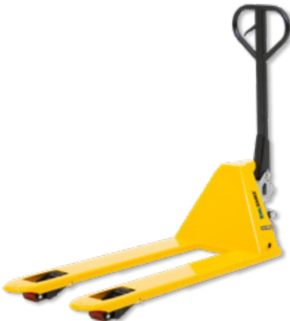
A low-profile pallet truck allows you to move pallets that are lower than the standard height of a EUR-pallet (100 mm). All palletised loads up to 2000 kg with low clearance opening can now easily be transported with use of this pallet truck. The minimum starting height is 52 mm. This model is often used on construction sites, e.g. to move bricks.
