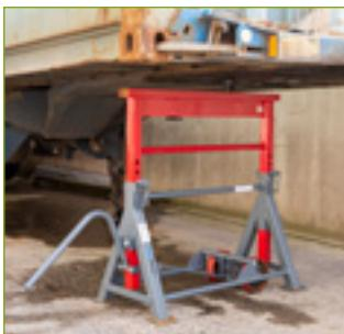
Thanks to the foldaway wheels, the safety trestle can easily be placed under the trailer to prevent it from tilting. The weight of the trailer is spread over the support to ensure stability. In this way, you can avoid damage to your truck, your goods and the surface. A safe environment guaranteed.
